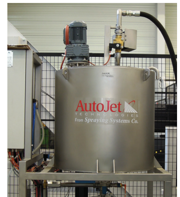
Base unit showing heated tank, inline heater and mixer
