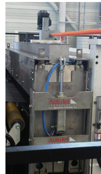
Coil Lubricator for 2.200 mm wide bands
