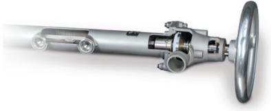
**Manual brush-type headers** scrub the interior wall of the header to prevent nozzle clogging. The brush operates without disruption to the system's process. The removed debris is evacuated through the flush-out valve.
