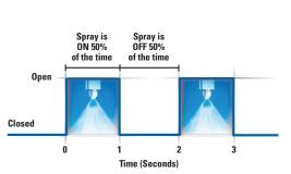
AutoJet Model 1550+ Modular Spray System enables Precision Spray Control, which dramatically increases turn-down ratios for low application rates and uniform coverage
