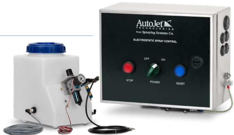
**The AutoJet ES250 Electrostatic Spray System** improves chain lubrication while greatly reducing oil consumption and conveyor downtime. The system is built around an AutoJet Spray Controller, electrostatic spray nozzles, a 16 liter (4.2 gallon) oil reservoir and a pressure regulator/filter/pressure switch. The system offers real-time monitoring of system parameters, including automated warning and alarm functions.
