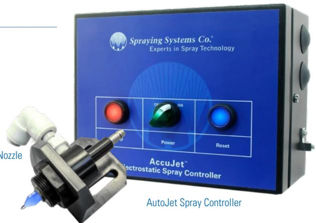
**Electrostatic spray technology** is based on the scientific principle that "opposites attract." In electrostatic spraying, a negatively charged liquid coating is attracted to a neutral, grounded target. The physical attraction of the liquid to the target pulls the coating to the chain surface, providing typical transfer efficiencies of greater than 90%. Overspray is eliminated, reducing clean-up and improving the work environment.
