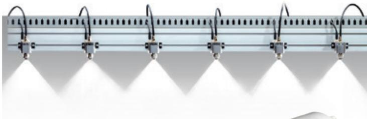
**PulsaJet® electrically-actuated spray nozzles** provide high-transfer efficiency to minimize waste and messy overspray. Cycle speeds up to 25,000 cycles per minute are possible to keep pace with fast line speeds. PulsaJet nozzles can be used with a variety of spray tips to ensure the performance matches the application requirements.
