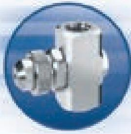
**J Series air atomizing nozzles** are available in many sizes and configurations. Inlet connections range from 1/8 to 1" with flow rates ranging from 0.55 to 906 gph at 40 psi (2.08 to 343 l/hr at 2.8 bar). Users can choose pressure- or siphon-fed spray set-ups and a round, wide-angle round, 360° circular, flat spray or deflected flat spray pattern.
