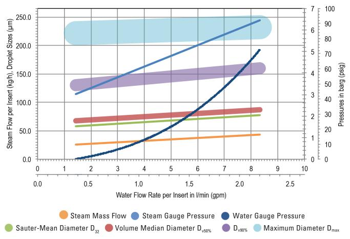
Data is based on spraying water under laboratory conditions using the Phase Doppler Interferometry (PDI). All values are to be computed utilizing the procedures for determing spray characteristics as outlined by ASTM (Standard E799).
