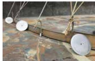
The required buoyancy is determined with the help of a tension gauge. After preparing the floats, they are attached to the rake using shackles and a chain. The length of the chains must be selected so that the floats swim above the sediments but do not get stuck in the solids floating on the surface of the water. A properly configured flotation system can double the lifespan of the heavy-duty wheels and significantly lower the expensive consequential damage on the bottom of the tank.
