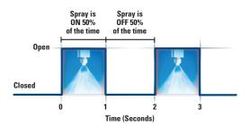
AutoJet Precision Lubrication provides automated spray control of nozzles to ensure precise, accurate placement of the oil on steel bars with minimal waste.
