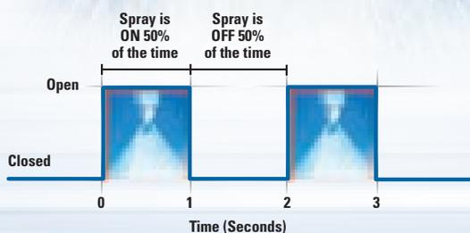
**Precision Spray Control (PSC)** involves switching spray nozzles on and off very quickly in order to control the flow rate. This cycling takes place so quickly that the flow often appears to be constant. PSC requires the use of electrically-actuated nozzles and an AutoJet spray controller.
