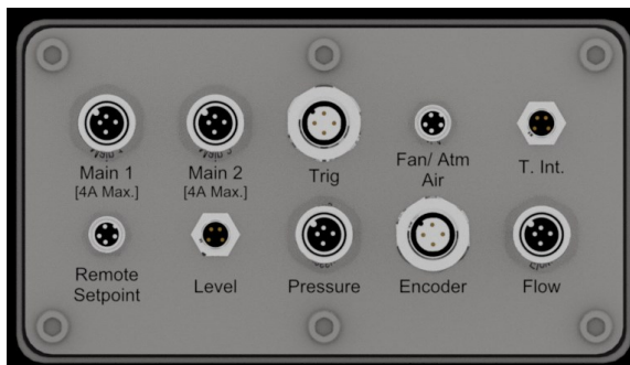
Channel A and Channel B bulkheads (bottom of 2150+)
