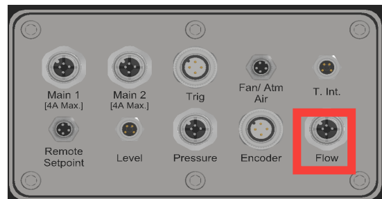
Plug and Spray connections, flow meter (located on bottom of 2150+)
