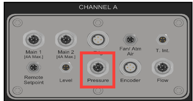
Plug and Spray connections, pressure sensor (located on bottom of 2150+)
