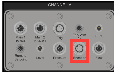
Plug and Spray connections, encoder (located on bottom of 2150+)
