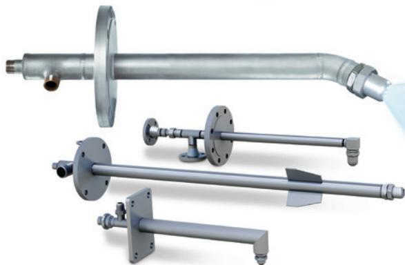
**Lances and Injectors.** We offer a full range of spray injectors. Our standard lightweight FloMax injectors are readily available in 0°, 45° and 90° configurations with quick-release or bolt-on flanges with optional adapters, cooling jackets, purge tubes and protective tubes
