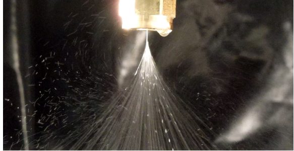
Figure 7. Electrostatic atomizer operating with d = 200\mu\text{m} , L/d = 1.0 , u_j = 10\text{m/s} and q_v = 2.2\text{C/m}^3 .
