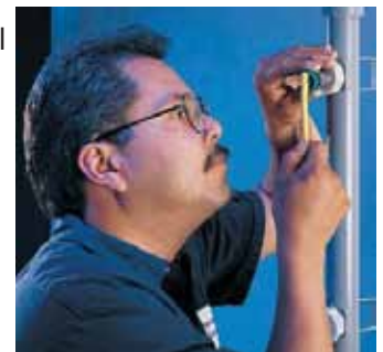
Clean nozzles with a material that is softer than the orifice, like a toothbrush or toothpick.
