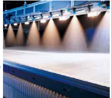
A Patterator measures spray distribution. The data is used to determine the optimal spray nozzle height and overlap in an application.
