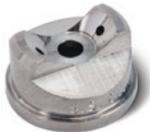
**External mix spray set-ups** produce a completely atomized spray by mixing the liquid and air outside the nozzle body. They are particularly useful when spraying viscous liquids. The SUE configuration shown here produces a flat spray pattern
