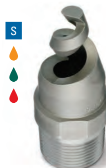
BSJ – 1/4" to 4" male conn. Threaded/Round or flat body style/stainless steel
