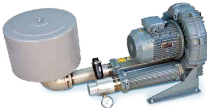
**Regenerative blowers** are rugged, reliable and require minimal maintenance. These blowers use a dynamic operating principle that recycles a certain amount of air and provide performance comparable to many multi-stage or positive displacement blowers.
