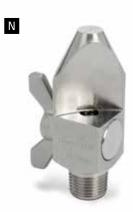
115220 RotoClean® **Clean-out Nozzle** 3/8" male conn. Flow rate below 7.7 gpm at 150 psi (29.15 lpm at 10 bar)
