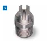
H-VV 1/8" to 1/4" male conn. Flow rates below 1 gpm at 40 psi (3.8 lpm at 2.8 bar)
