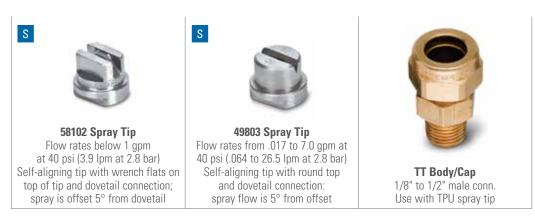
Dovetail spray tips can be used on a variety of body types. Please contact your sales engineer for body options and dimensions.
