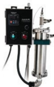
**In-line Heater** provides heat on demand to warm the release oil up to 130°F (54°C) just prior to spraying to improve coating uniformity and minimize the risk of clogging.
