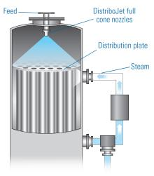
DistriboJet nozzles have large flow passages and large open orifices to assure non-clogging operation. The operating range is 1 to 60 psi (.07 to 4 bar) with a full cone spray pattern developing at 1 psi (.07 bar).
