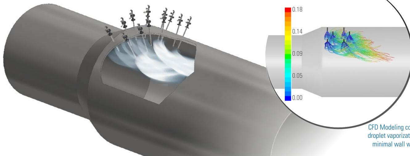
CFD Modeling confirmed droplet vaporization with minimal wall wetting
