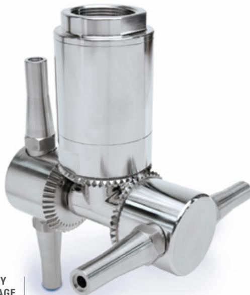
**The TankJet 65 tank cleaner** includes four solid stream nozzles that feature slow, steady, multi-axis rotation and a tight, 360° indexing pattern that covers the tank every 45 revolutions and provides excellent dwell time on tank surfaces
