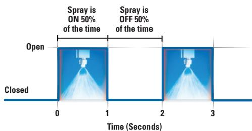
**Precision Spray Control (PSC)** turns electrically actuated PulsaJet nozzles on and off quickly to control flow rate. With traditional nozzles, flow rate adjustments require a change in liquid pressure, which also changes the nozzle's spray angle/coverage and droplet size. With PSC, pressure remains constant, enabling flow rate changes without affecting spray performance. This reduces the use of costly coatings by applying the proper volume directly on the cables.
