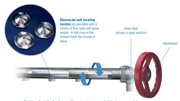
**An internal rotating brush assembly** scrubs the interior wall of the shower as well as each disc-type shower nozzle orifice. In just a few seconds, debris is swept away through the flush-out valve, restoring full liquid flow to the system without contaminating the sprayed surface. And, there's no need to stop the system. The brushes operate without disruption to normal processes.
