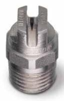
**VeeJet® nozzles** produce a thin, tapered-edge, rectangular spray pattern with medium sized drops and higher impact. Positioned to the side of the rail cars, the higher impact spray penetrates the falling iron ore and provides effective dust control.
