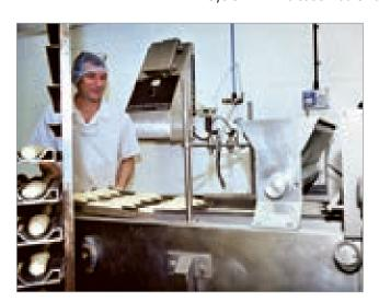
to conveniently set the delay time between detection of the leading edge of the baking tray and when the nozzles spray. The duration of the spray time for various baked goods is also easily set. Accurate control of these operating parameters ensures precise coverage of the rolls every time.
