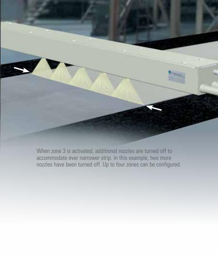
When zone 3 is activated, additional nozzles are turned off to accommodate ever narrower strip. In this example, two more nozzles have been turned off. Up to four zones can be configured.
