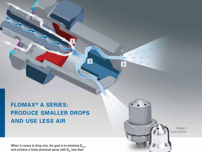
100 microns at 10 gpm (37.8 lpm). This drop size cannot be achieved with a single-step atomization process.
