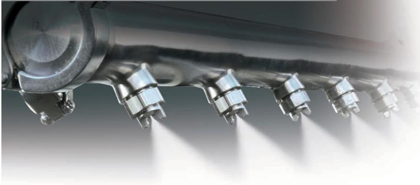
The **63600 spray manifold** provides superior performance with viscous coatings. The large diameter liquid passage helps to ensure consistent flow and minimize pressure drop while the hot water jacket improves flow and maintains a consistent temperature up to the nozzle orifice. The 63600 spray manifold also has a sanitary design to reduce the risk of contamination.
