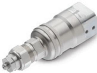
**Electrically-actuated spray nozzle** provides continuous spraying or high-speed cycling up to 2,000 cycles per minute. All connections are located at the rear of the nozzle to minimize the nozzle profile. The mounting and connections are not disturbed during maintenance because of a quick-change fluid module for replacing wear parts.
