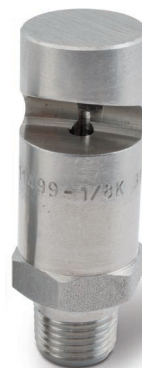
11499 & 13063 1/8" male conn. Flow rates below 4.4 gpm at 60 psi (16.7 lpm at 4.1 bar)
