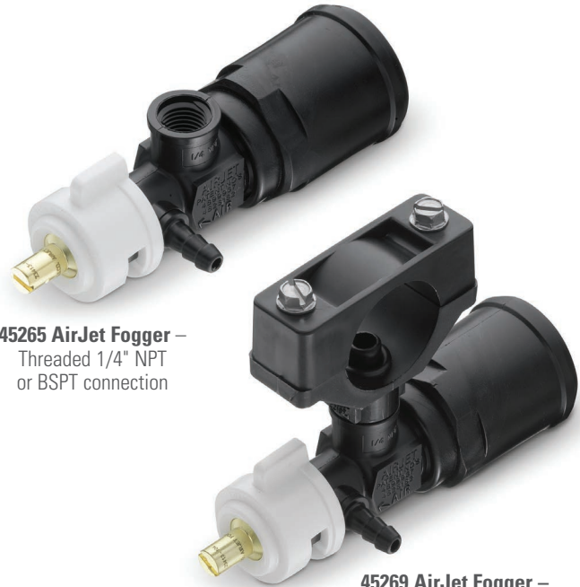
45269 AirJet Fogger – Split-eyelet design provides fast installation of the nozzle onto the liquid supply pipe. No additional pipe fittings are required. Pipe cutting, threading and brazing are eliminated.
