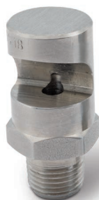
K 1/8" to 1" male conn. Flow rates below 110 gpm at 60 psi (410 lpm at 4.1 bar)
