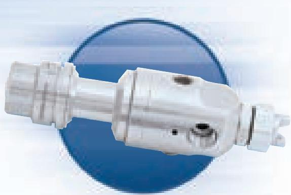
**Three JAUMCO automatic air atomizing nozzles,** triggered by a photoelectric sensor that detects the presence of bread pans, coat uniformly without overspray. The nozzles feature an internal air cylinder for controlled on/off operation up to 180 cycles per minute. The cycling of the nozzle interrupts only the liquid portion of the spray to prevent dripping.
