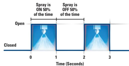
**AutoJet Precision Lubrication** provides automated spray control of nozzles to ensure precise, accurate placement of the oil on steel bars with minimal waste.
