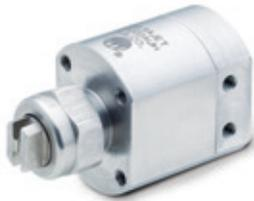
**Pulsajet® electrically-actuated spray nozzles** provide high transfer efficiency to minimize waste and messy overspray. Cycle speeds up to 25,000 cycles per minute are possible to keep pace with fast line speeds. Pulsajet nozzles can be used with a variety of spray tips to ensure the performance matches the application requirements.
