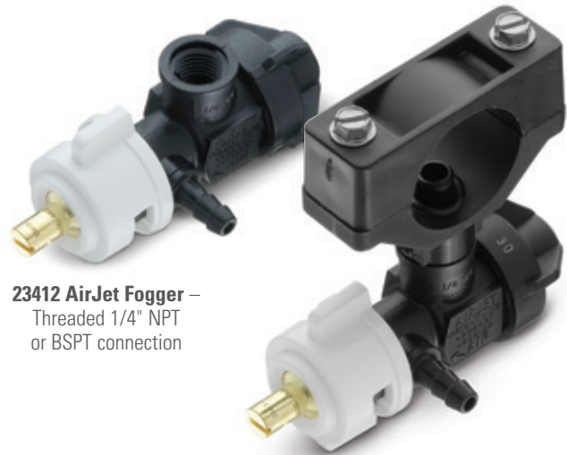
QJ25655 AirJet Fogger – Split-eyelet design provides fast installation of the nozzle onto the liquid supply pipe. No additional pipe fittings are required. Pipe cutting, threading and brazing are eliminated.
