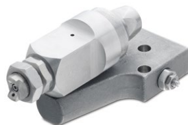
19330-1/4JAUPM – Plate-mounted nozzle with all inlet connections at the rear of the mounting plate. Locking regulating screw allows precise adjustment of atomizing air
