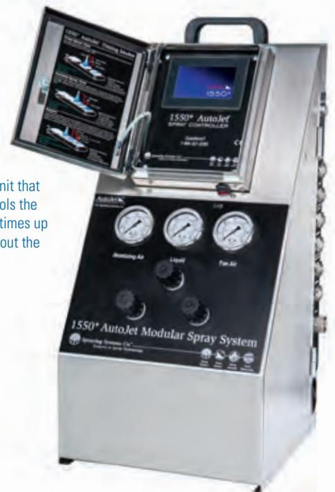
**Precision Spray Control (PSC)** turns nozzles on and off quickly to control flow rate. This cycling is so fast that the flow often appears to be constant. Unlike traditional nozzles, which require a change in liquid pressure, PSC allows the pressure to remain constant and enables flow rate changes without changing the spray angle or drop size.
