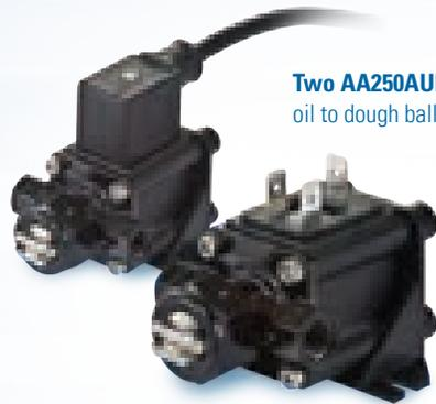
Two AA250AUH hydraulic automatic nozzles apply oil to dough balls as they pass under the spray manifold.
