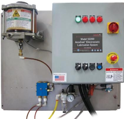
**The patent-pending Model 52200 AutoJet Electrostatic Lubrication System** improves chain lubrication while greatly reducing oil consumption and conveyor downtime. The system is built around an AutoJet Spray Controller, electrostatic spray nozzles, a 16 liter (4.2 gallon) oil reservoir and a pressure regulator/filter/pressure switch. The system offers real-time monitoring of system parameters, including automated warning and alarm functions.
