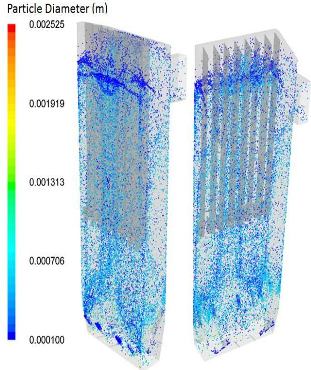
**Figure 7.** Solid Phase Particulate Distribution Colored by Diameter in CFB Boiler
