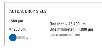
Liquid properties, nozzle capacity, spraying pressure and spray angle also affect drop size. Lower spraying pressures provide larger drop sizes. Conversely, higher spraying pressures yield smaller drop sizes. Within each type of spray pattern the smallest capacities produce the smallest spray drops, and the largest capacities produce the largest spray drops.
