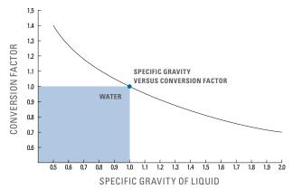
KEY: Conversion factor multiplied by the capacity of the nozzle when spraying water gives the capacity of the nozzle when spraying a liquid with a specific gravity corresponding to the conversion factor. This conversion factor accounts only for the effect of specific gravity on capacity and does not account for other factors affecting capacity.
