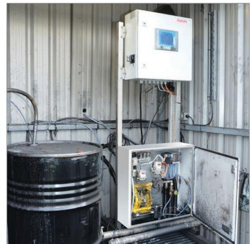
Four D55500 air atomizing nozzles apply lubricant to the die. At right, the control panel with touch screen HMI is seen.
