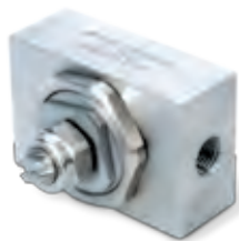
AA10000AUH-72440-1/4 Jacketed design keeps nozzle and sprayed liquid at a consistent temperature Typical flow range: 0.0017 - 0.47 gpm (0.006 - 1.8 lpm) Electropolished or chromium nitride coated magnetic stainless steel, stainless steel, Viton or EPDM seals, PPS and PEEK Up to 15,000 cycles per min
