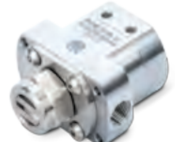
AA10000AUH-104215 Front port for liquid recirculation Typical flow range: 0.0017 - 0.47 gpm (0.006 - 1.8 lpm) Stainless steel, Viton or EPDM seals, PPS and PEEK Up to 15,000 cycles per min
