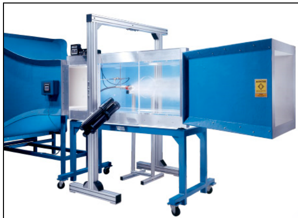
Figure 1. PDPA mounted with wind tunnel
