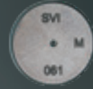
Worn Orifice Competitor: 20% increase in flow rate
