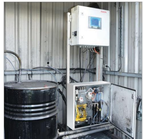
Four D55500 air atomizing nozzles apply lubricant to the die. At right, the control panel with touch screen HMI is seen.
