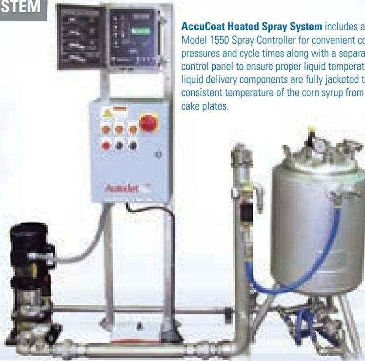
**AccuCoat Heated Spray System** includes an AutoJet® Model 1550 Spray Controller for convenient control of spray pressures and cycle times along with a separate heater control panel to ensure proper liquid temperature. All liquid delivery components are fully jacketed to maintain consistent temperature of the corn syrup from tank to the cake plates.
